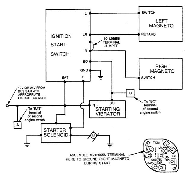
A & B For twin engine installations, starting vibrator may be shared by interconnecting ignition/start circuits at points shown.
