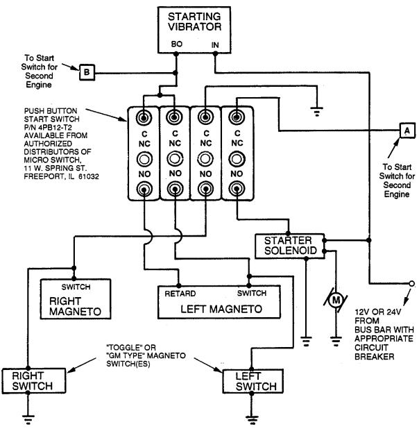
A & B For twin engine installations, starting vibrator may be shared by interconnecting ignition/start circuits at points shown.
