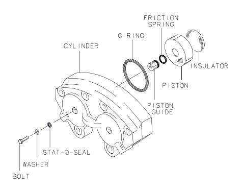
Figure 302 - Internal Piston Guide
