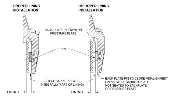
Figure 201 - Pin Installation, Metallic Lining
