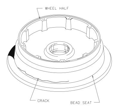
Figure 308 - Bead Seat Inspection
