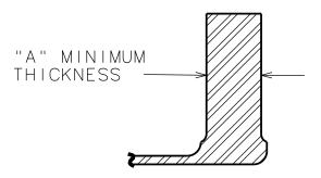
Figure A2 - Disc Thickness Measurement
