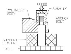
Figure 305 - Anchor Bolt Installation
