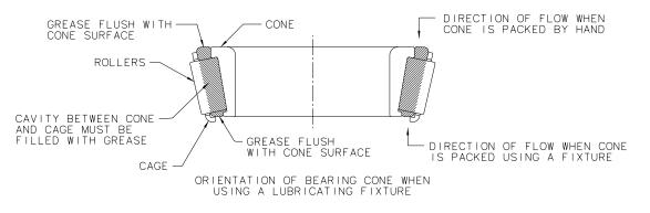
Figure 313 - Packing Bearing Cones
