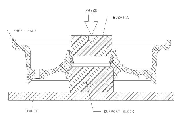
Figure 311 - Bearing Cup Installation
