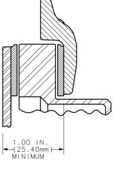
Figure A1-1 Disc Wear Measurement (Piper Aztec)
