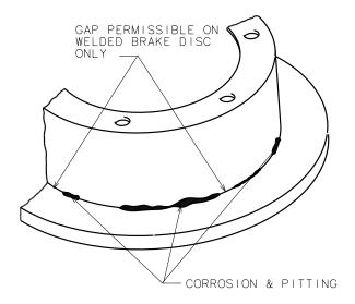
Figure 310 - Disc Inspection
