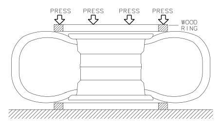
Figure 306 - Tire Removal
