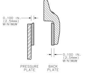
Figure A1 Minimum Lining Thickness
