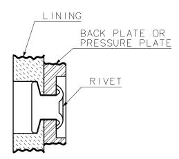
Figure 202 - Rivet Installation, Organic Lining
