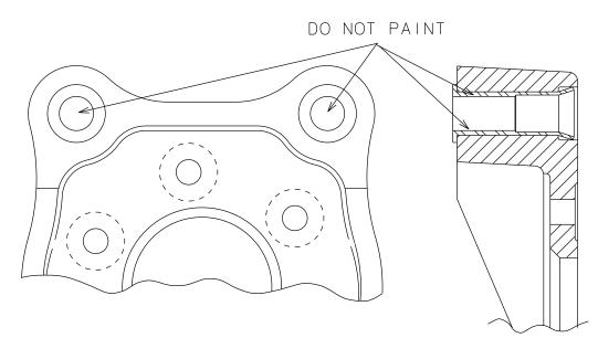
Figure 314 - Typical Torque Plate (Cast), Painted Surfaces
