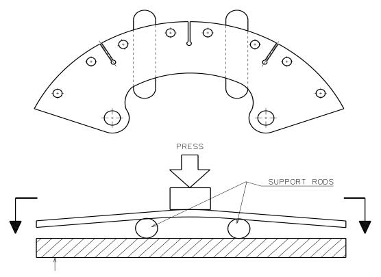
Figure 203 - Pressure Plate Straightening
