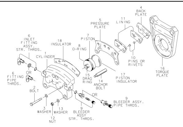
Figure 2 - Typical External Disc Brake Assembly
