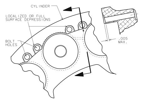
Figure 304 - Cylinder To Back Plate Surface Inspection
