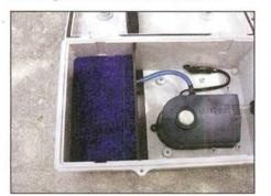
the crankcase and replacing it with moisture-free air. The idea has enough credence for three companies to have introduced dehydrator products. The latest comes from Tempest/Aero group, which adds a dehydrator to its well-regarded line of dry vacuum pumps and oil filters. The AA1000 Engine Preservation Systems retails for \$235.
