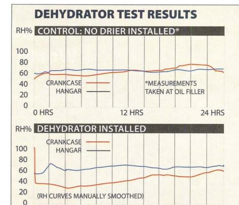
To test the Tempest dehydrator, the engine was flown to warm the oil to normal operating temperature. We then installed the product according to the manufacturer's instructions. Temperature, humidity and dewpoint data was sampled using Lascar programmable dataloggers. Data were sampled from the oil filler neck with the sensor inserted through a tightly sealed foam gasket. For this test, only relative humidity is plotted.
